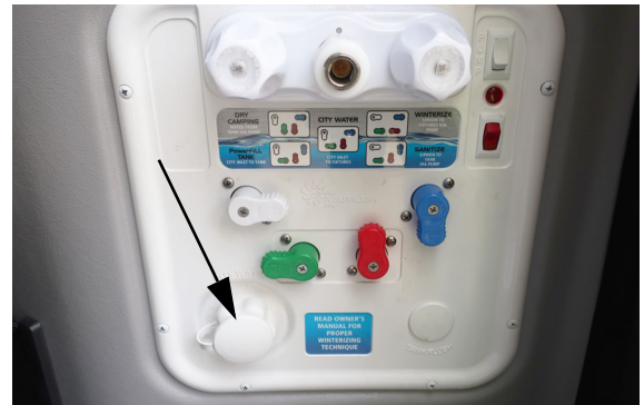
Tank Fill Inlet (Located behind the passenger rear door) -Typical View
