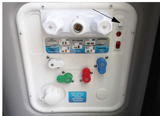
Pump switch -Typical View
