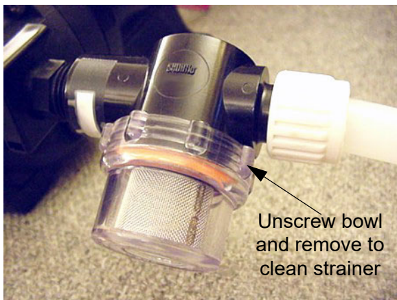
Water Pump Strainer -Typical View
