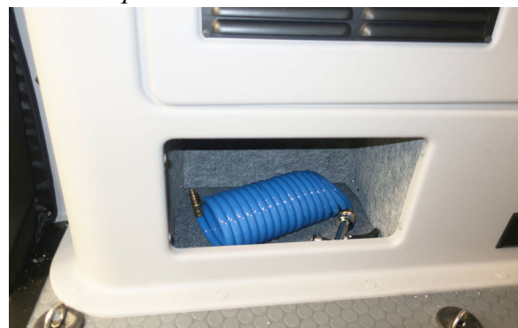
Exterior Shower Hose (located behind rear driver’s side door, left storage compartment - Typical View)
